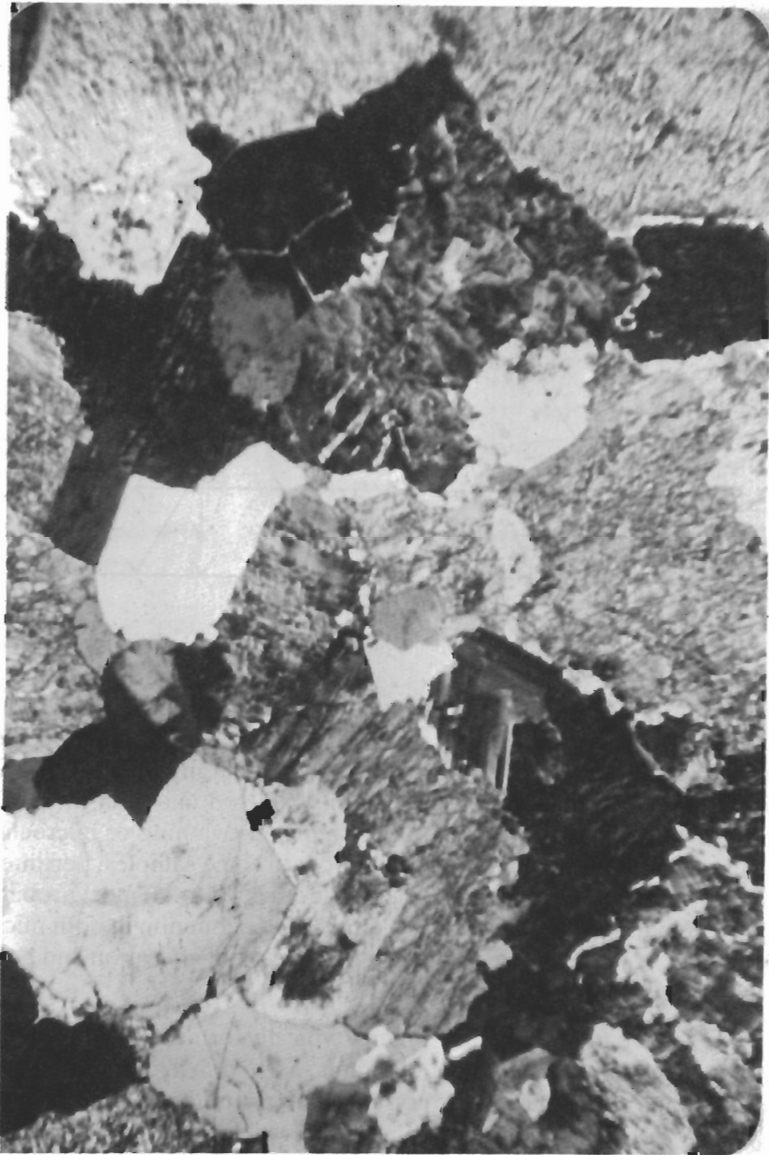
FIG. 4. Photomicrograph showing the dominance of perthites in the Dariyah granite (scale \times 25 ).
